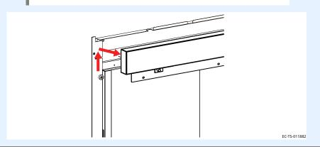
4. **Secure** the warmer to the wall using the two (2) self-tapping wall screws (SC-47298) ② and a #3 Phillips screwdriver.
