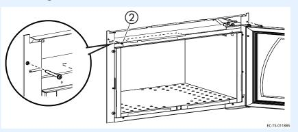
5. **Re-install** the interface assembly. **Make sure** all of the tabs lock the interface bends into place.
