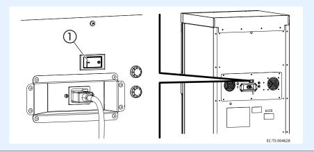
2. **Press** the ON/OFF button . The screen turns on.
